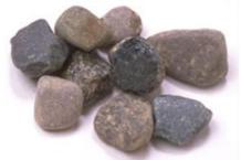
Worn River Gravel (G-699): 9.5 to 15.9 mm (3/8 to 5/8 in), Standard Michigan; used in SAE J400 and ASTM D-3170
